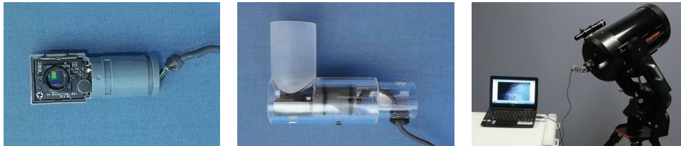
Figure 1. Camera and telescope. Left: The lens and much of the casing is removed from an ordinary webcam. Center: KPU Mk II camera. The new packaging fits the eyepiece holder of telescopes. Right: An 8-inch telescope equipped with a KPU Mk II camera controlled by a netbook computer.
